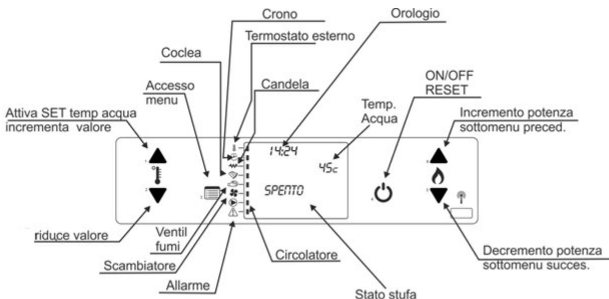
Below is a list of meanings of LEDs found on control panels:
