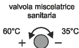
**At the back of the boiler the mixing valve knob can be accessed to adjust the temperature of the outgoing hot water (see fig. 14.)**
